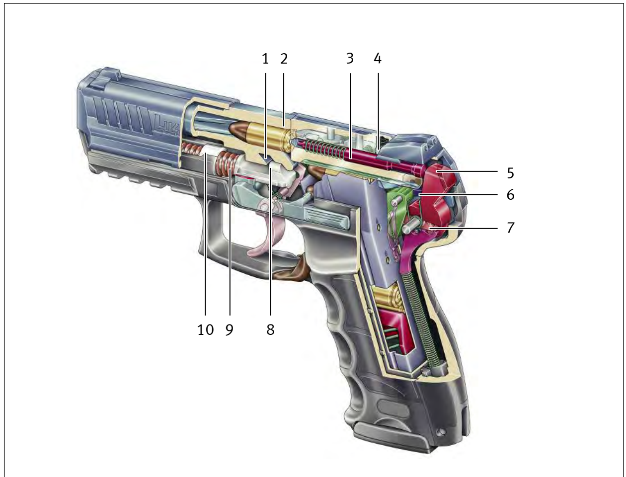
Fig. 13a: CDA trigger variant, cutaway view
