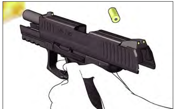
Fig. 33b: Path of the slide
