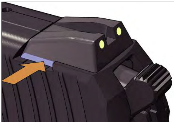
Fig. 28a: Lateral shifting of the rear sight
